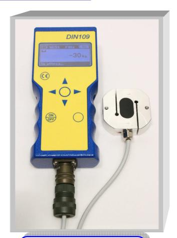
Dynamometer DIN109 is available with a large catalogue of load cells
